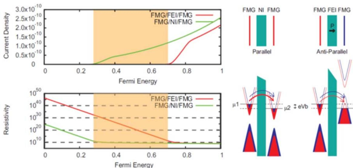
Fig. 1. Emergence of giant resistance in FMG/FEI heterojunctions. The blockade of quantum tunneling through the heterojunction originates from the anti-parallel configuration of FMGs.
